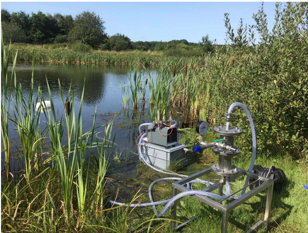
Figure 19. Equipment for sampling of water in a stormwater pond. Photo from Liu et al (2019).
