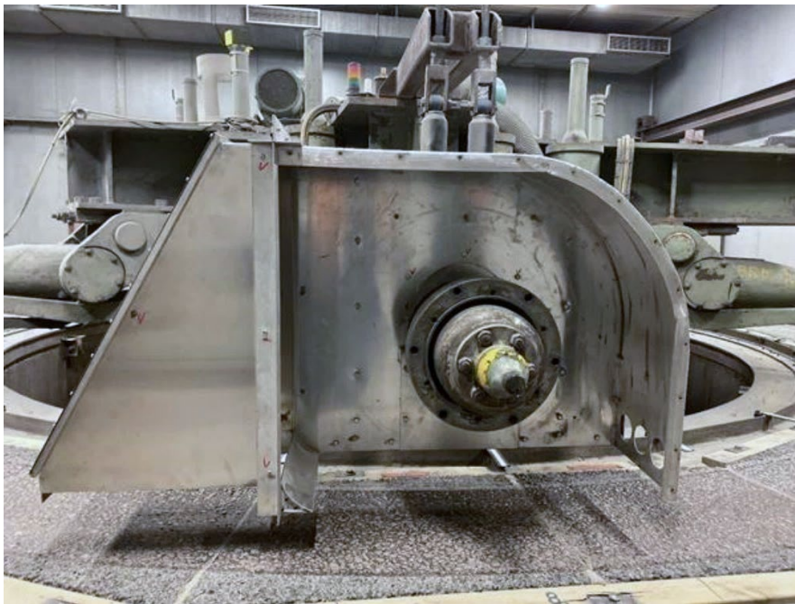
Figure 9. Collection device for VTI's road simulator, used to collect particles from tyre and road surface wear. Photo: Mats Gustafsson, VTI.
