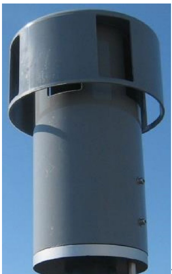
Figure 15. Sigma-2 passive sampler for airborne particles. Photo: Particle Vision.
