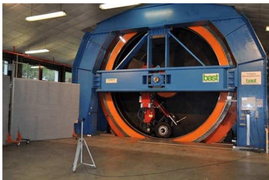
Figure 7. Vertical drums for testing of tyres in contact with road surfaces. BASt (Bundesanstalt für Straßenwesen) Germany. Photo: Re-tyre project, EU.
