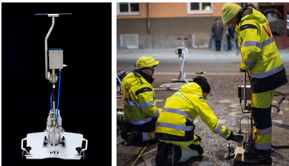
Figure 11. Wet Dust Sampler (WDSII), Left: sampling device. Right: field sampling. Photo: Mats Gustafsson, VTI and Sami Kulovuori, Metropolia.
